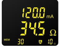
Indicates voltage/current alarm threshold along with the direction of impedance
